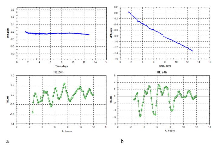
Fig.6 Frequency and TIE measurement for quartz oscillator a)without and b)with "short-term" frequency changes
