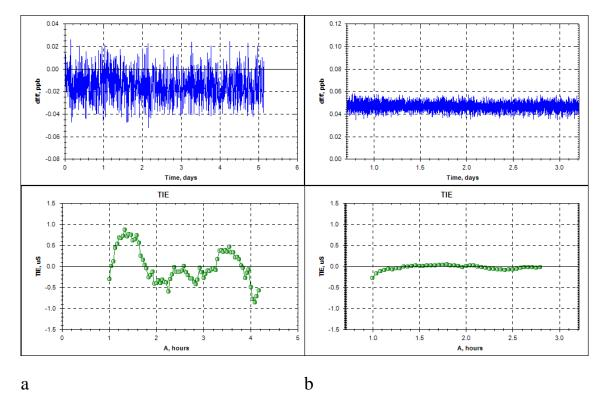
Fig.4 Measurement of frequency and TIE estimation for rubidium oscillator a) before and b) after implementation of the above measures to prevent mutual syntonization of frequency.
