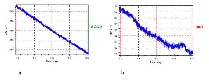
Fig.5 Figure 5a aging curve satisfactory for TIE of 100...400 ns requirement. Figure 5b shows "standard" aging curve.
