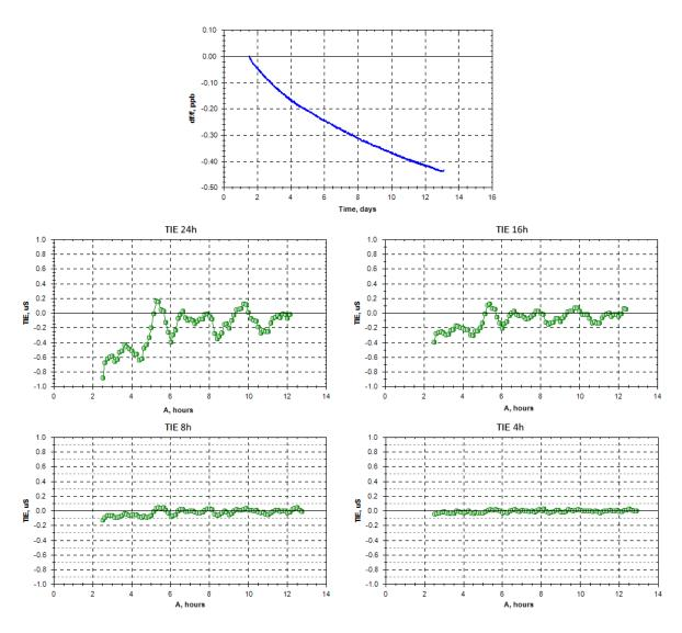
Fig. 7 Measurement of TIE per 4, 8, 16 and 24 hours
